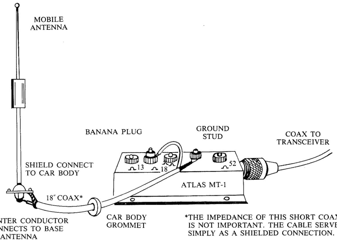
**INSTALLATION:** The MT-1 transformer is weather sealed and has a black anodized aluminum case, but even so it is recommended that it be installed inside the car body. In cases where the antenna is mounted on a rear bumper mount, install the transformer in the trunk compartment and drill a 3/8 inch hole for a rubber grommet to pass the short length of coax. from the antenna base to the transformer. This is the piece of coax. provided with the transformer, and has a banana plug on one end.
