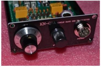
[ ] Preset the IF GAIN control to mid-way and you are ready to start alignment. After alignment, remember to install the top chassis using another 4x black chassis screws.
