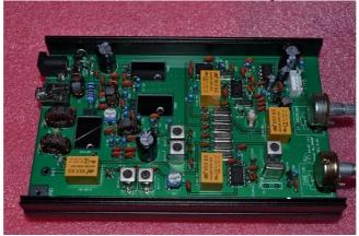
[ ] Bend the pins of the 7808, IRF640, and D882 (IRF530 for 20m version) semiconductors as shown. Please note that IRF640 (IRF530 for 20m version) is a electrostatic sensitive part, so handle it with care.
