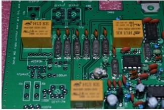
[ ] Plug in a 12~13.8 V power supply and connect an external speaker to the speaker connector. Touch pin 5 of the uninstalled NE602A using tweezers to note a little noise from the speaker. If it is not normal, please check your soldering. If it is okay, disconnect the power supply and the external speaker to proceed to the next step.
