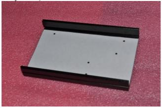
[ ] Drill 7x M3 holes. The locations for the 4x chassis feet holes are not very important, but you have to be very careful with the locations of the holes for the three semiconductors. Please pay close attention while you are drilling. After you are done with the drilling, please make sure you remove the blurs from the holes.
