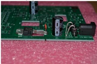
[ ] Plug in a  $12\sim13.8$  V power supply and measure the voltage on pin 3 of 7808 near to the 104 capacitor to see if it is within  $\pm -5\%$  of 8 V; if not, check power supply polarity and your soldering [ ] Disconnect the power supply and proceed to the next step.
