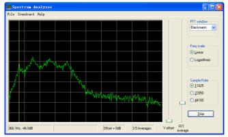
Remove the audio cable and connect an external speaker. Use band noise or a signal to peak again the RX BPF. If you hear strong broadcast interference, especially at night time, you may need to turn the RF ATT trimmer clockwise until the interference is gone. If you attenuate too much, the
