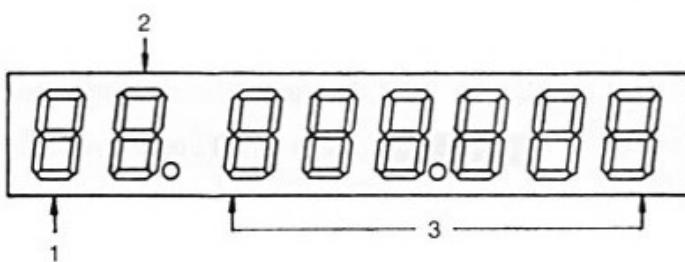
1. The **channel digit** shows the number of the channel under scanning, monitoring or programming.
