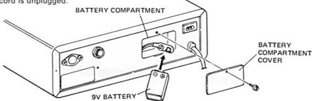
**NOTE:** To avoid loss of the program memory, keep the receiver connected to an AC or DC power source when replacing the battery. Replace the battery at least every six months.
