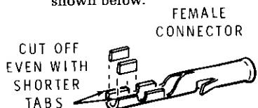
(✓) 2. Install a 1" bare wire into a female connector as shown.
