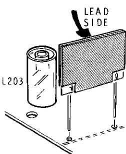
(✓) Prepared RF shield. Solder the leads to the foil and cut off the excess lead lengths.
