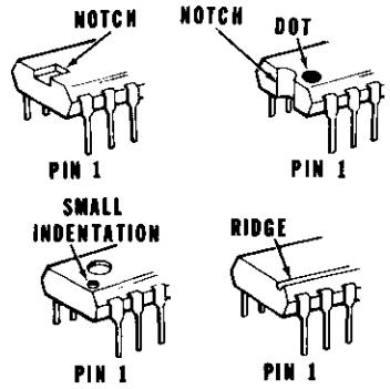
Be sure you install each IC so its pin 1 end is toward the index mark on the circuit board.
