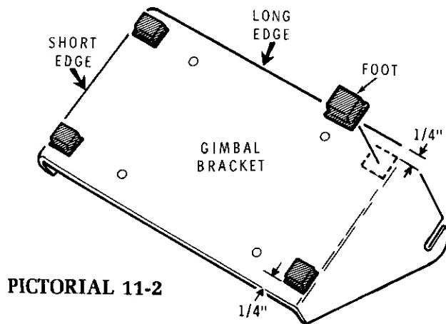
Refer to Pictorial 11-2 and turn the bracket upside down as shown. Then remove the paper backing from each of the feet and press them into place on the underside of the bracket. Be sure to keep  $1/4"$  distance between the sides of the feet and the longer sides of the bracket, as shown. The edges of the feet should be flush with the shorter edges of the bracket.
