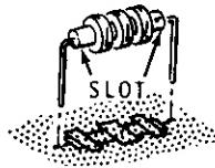
(✓) RFC201: 350  $\mu$ H choke (#45-82). Mount this choke so its body is 1/16" above the circuit board.
