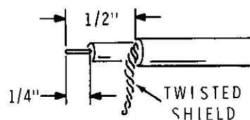
1. Remove 1/2" of the outer insulation.
