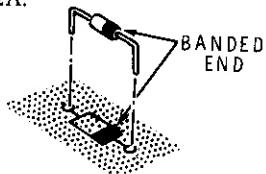
(✓) VD501: FV1010 diode (#56-77). Solder the leads to the foil and cut off the excess lead lengths.
