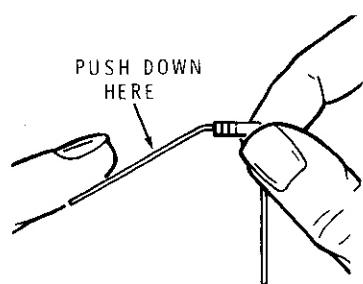
✓) Push the leads through the holes at the indicated location on the circuit board. The end with color bands may be positioned either way.
