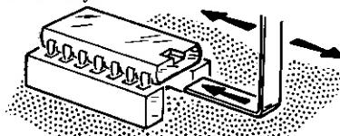
Push the shorter end of the lifter in between the IC and the socket and rock the longer portion back and forth. Be very careful, as the IC pins are very easily bent.
