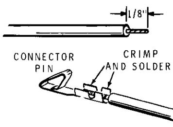
NOTE: When you perform the following step, be sure to position the connector housing and connector pins as shown before you insert the pins into the housing. Push in on the wire until the pin snaps into place.
