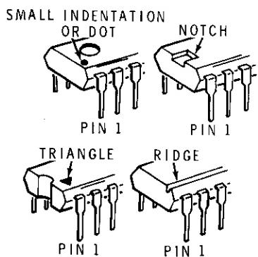
(✓) IC502: MC1648P integrated circuit (#443-740). Position the pin 1 end of the IC over the index mark on the circuit board as shown. Then insert the pins into the circuit board and solder them to the foil. Do not solder the leads that do not have foil.
