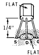
Install seven MPSA20 transistors (#417-801) at the following locations:
