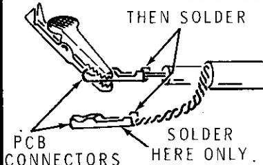
1. Place the end of the shield lead in a PCB connector. Then crimp the connector around the lead.
