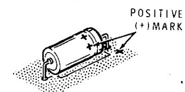
(✓) Solder the leads to the foil and cut off the excess lead lengths.
