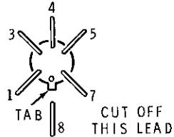
(✓) IC201: UA703 IC (#442-20). Position the tab on the IC over the outline of the tab on the circuit board. Then insert the leads in the corresponding holes in the circuit board. Position it 1/4" above the circuit board. Then solder the five leads to the foil and cut off the excess lead lengths.
