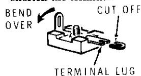
NOTES: In the following steps, as you install each trimmer capacitor, solder its terminals to the foil side of the circuit board as follows:
