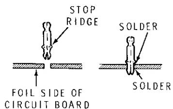
(✓) Install 12 small PCB pins (#432-121) in holes A through M.
