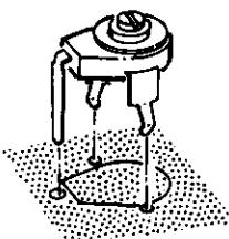
(V) L501: .165  $\mu$ H coil (#40-1907). Install the coil so the tab is positioned as shown on the circuit board. Hold this coil down tightly against the circuit board while you solder the leads to the foil. Then cut off the excess lead lengths.
