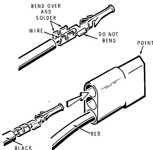
NOTE: In the following steps you will install a connector on the output wires of the Heathkit power supply for this Transceiver. The output has one red (positive) and one black (negative, or ground) wire.
