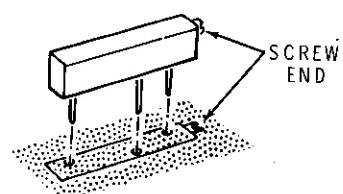
(✓) R126: 100 kΩ control. Solder the lugs to the foil and cut off the excess lug lengths.
