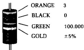
$$30 \times 100,000 = 3,000,000 \Omega \text{ (or } 3 M\Omega\text{)}$$
