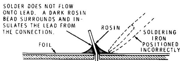
When the lead is not heated sufficiently, the solder will not flow onto the lead as shown above. To correct, reheat the connection and, if necessary, apply a small amount of additional solder to obtain a good connection.
