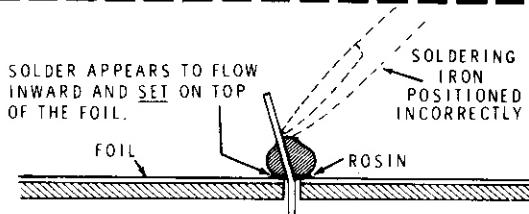
When the foil is not heated sufficiently the solder will blob on the circuit board as shown above. To correct, reheat the connection and, if necessary, apply a small amount of additional solder to obtain a good connection.
