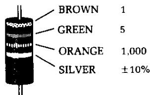
$$15 \times 1,000 = 15,000 \Omega \text{ (15,000 OHMS), or "15 k}\Omega\text{"}$$
