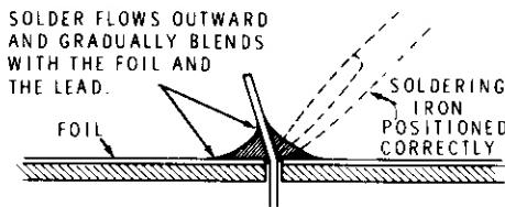
When you heat the lead and the circuit board foil at the same time, the solder will flow evenly onto the lead and the foil. The solder will make a good electrical connection between the lead and the foil.
