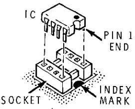
(✓) IC101: MC1458 integrated circuit (#442-21).
