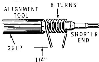
(3) Form the two coil leads so they point straight down as shown.
