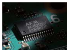
AD/DA converter ADC Signal/(Noise+Distortion): 10 dB ADC Dynamic range, S/N: 133 dB DAC Signal/(Noise+Distortion): 97 dB DAC Dynamic range, S/N: 115 dB
