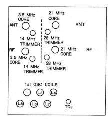
Reference: Layout of ANT. and RF Coitrimmers in RF Unit UC-1117J.
