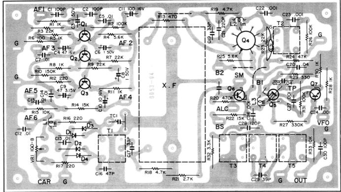
Q1:2SC871(E), Q2,3:2SC733(Y.GR), Q4:TA7045M, Q5:3SK22(GR), Q6:2SA495(Y), Q7:2SC460(B), D1~4:1N60
