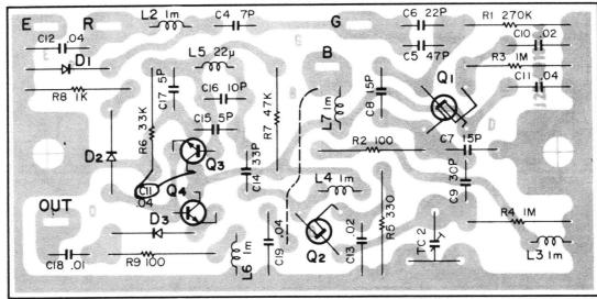
Q1:3SK22(Y), Q2:2SK19(Y), Q3,4:2SC46O(B), D1:SD111, D2,3:1N6O
