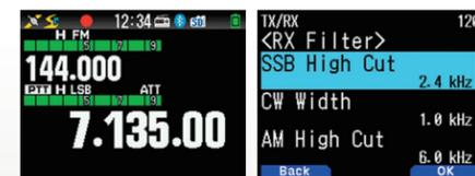
HF band SSB reception (PTT icon displays operating band) IF receiving filter settings
