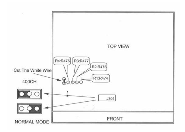
Radio starts up in mode "RU".(400CH and 15W) You can not switch anymore to other standards like EU, EC or PL etc unless you delete this modification by putting jumper in original position again!!
