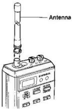
Your scanner's antenna jack makes it easy to use your scanner with a variety of antennas. You can remove the supplied antenna and attach a different one, such as an external mobile antenna, telescopic antenna, or outdoor base antenna. Radio Shack stores sell the antenna connector adapters that let you use these antennas.
