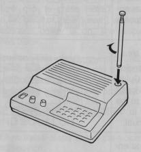
The telescoping antenna is adequate for strong local signals, but for best results, attach a multi-band outdoor antenna to the scanner. Your local Radio Shack store sells a complete line of outdoor scanner antennas. To install an outdoor antenna, do the following:
