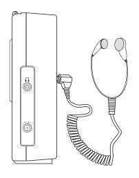
The socket for the headphones , which is suitable for a cinch plug of 3.5mm diameter, is marked with the headphone symbol.
