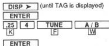
The alphanumeric tag can store up to 7 characters of letters and/or numerals. To enter a tag into the display, select the TAG display using
