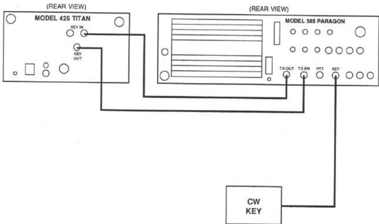
FIGURE 5-7. QSK HOOK-UP WITH TITAN AMPLIFIER
