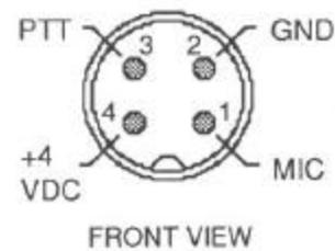
**FIGURE 3-2. MIC CONNECTIONS**
