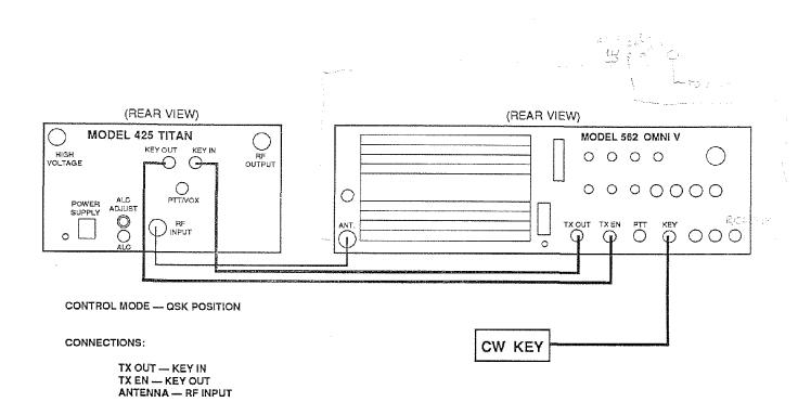
FIGURE 5-9. QSK HOOK-UP WITH TITAN AMPLIFIER
