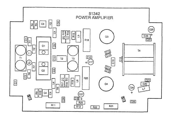
FIGURE 6 - 46. 81342 RF POWER AMPLIFIER COMPONENT LAYOUT
