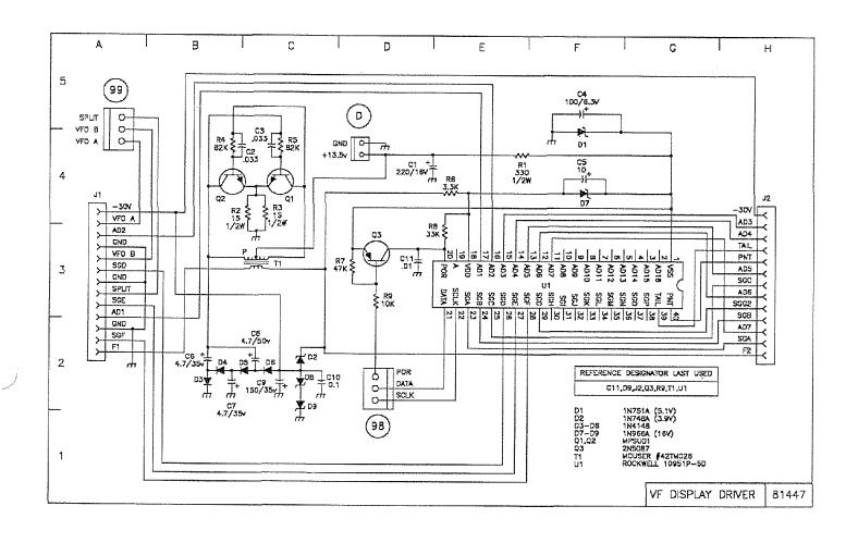
FIGURE 6-58. 81447 VF DISPLAY DRIVER BOARD SCHEMATIC
