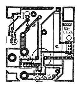
FIGURE 6-62. 81328 DC POWER BOARD CIRCUIT TRACE
