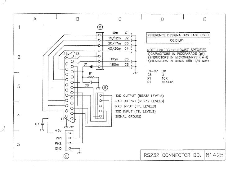
FIGURE 6-70. 81425 RS232 CONNECTOR BOARD SCHEMATIC
