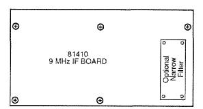
FIGURE 5-3. 9 MHZ IF CRYSTAL FILTER OPTION
