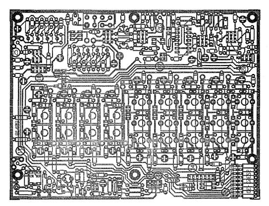
FIGURE 6-5. 81409 BAND PASS FILTER CIRCUIT TRACE
