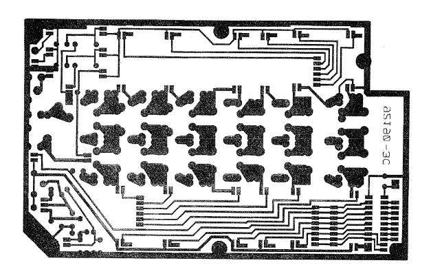
FIGURE 6-2. 81455 TRANSMIT LOW PASS FILTER CIRCUIT TRACE
