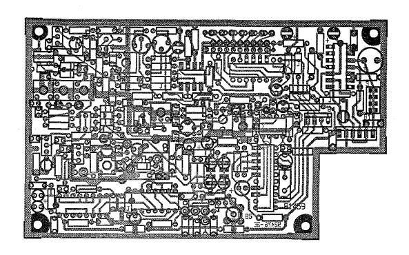
FIGURE 6-21. 81459 5.0-5.5 MHZ PLL BOARD CIRCUIT TRACE
