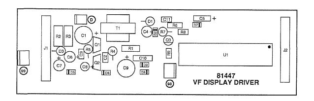
FIGURE 6-57. 81447 VF DISPLAY DRIVER BOARD COMPONENT LAYOUT
