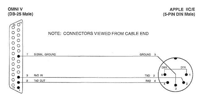
FIGURE 5-10D. APPLE IIC/E RS232 CONNECTOR CABLE
