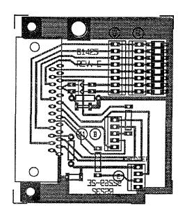
FIGURE 6-68. 81425 RS232 CONNECTOR BOARD CIRCUIT TRACE
