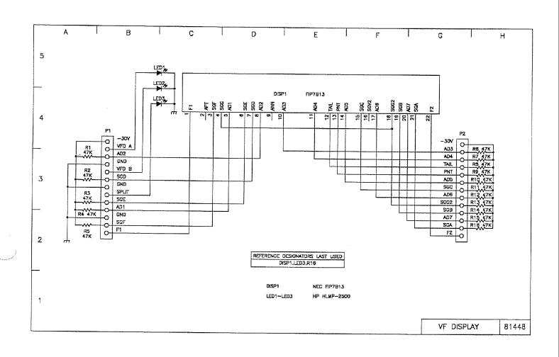
FIGURE 6-61. 81448 VF DISPLAY BOARD SCHEMATIC
