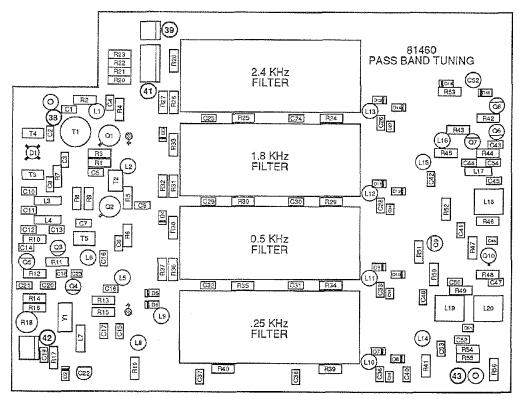
FIGURE 6-15. 81460 PASS BAND TUNING BOARD COMPONENT LAYOUT
