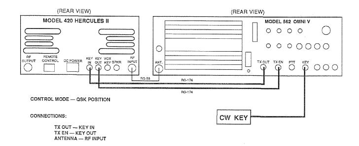
FIGURE 5-8. QSK HOOK-UP WITH HERCULES II AMPLIFIER
