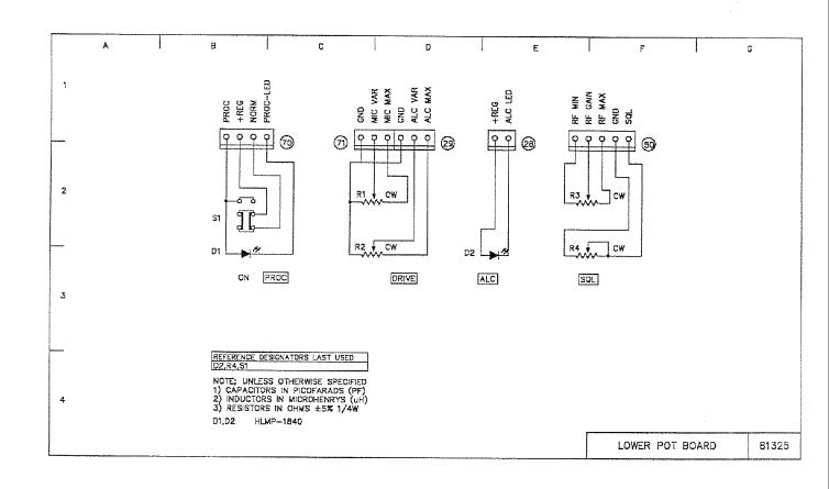
FIGURE 6-35. 81325 LOWER POT BOARD SCHEMATIC
