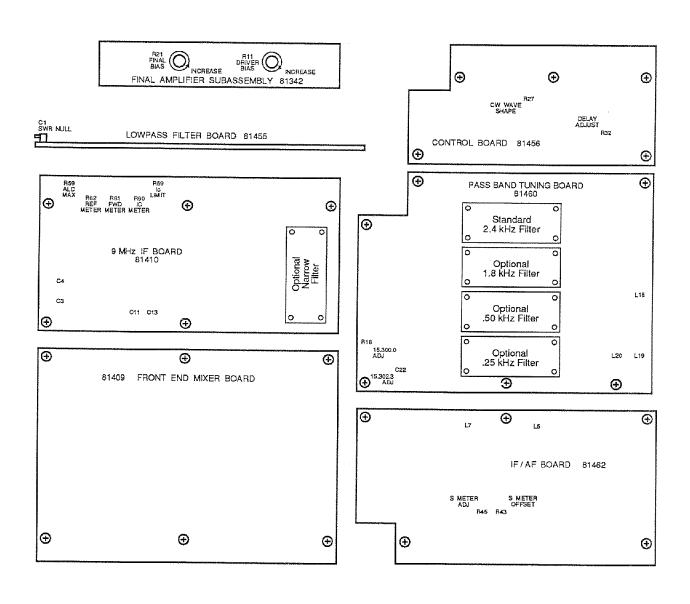
FIGURE 5-5. MODEL 562 ADJUSTMENTS (BOTTOM VIEW)
