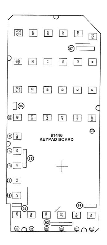
FIGURE 6-54. 81446 KEYPAD BOARD COMPONENT LAYOUT
