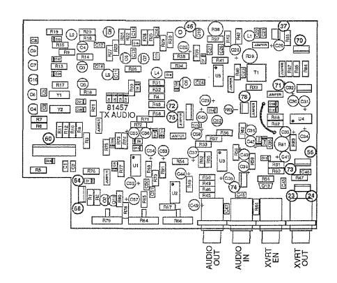
FIGURE 6-40. 81457 TRANSMIT AUDIO/BFO BOARD COMPONENT LAYOUT
