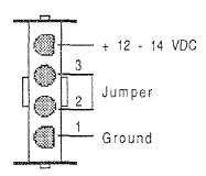
FIGURE 1-1. POWER SUPPLY CONNECTIONS
