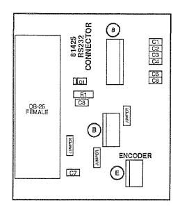
FIGURE 6-69. 81425 RS232 CONNECTOR BOARD COMPONENT LAYOUT
