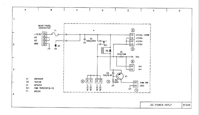
FIGURE 6-64. 81328 DC POWER BOARD SCHEMATIC
