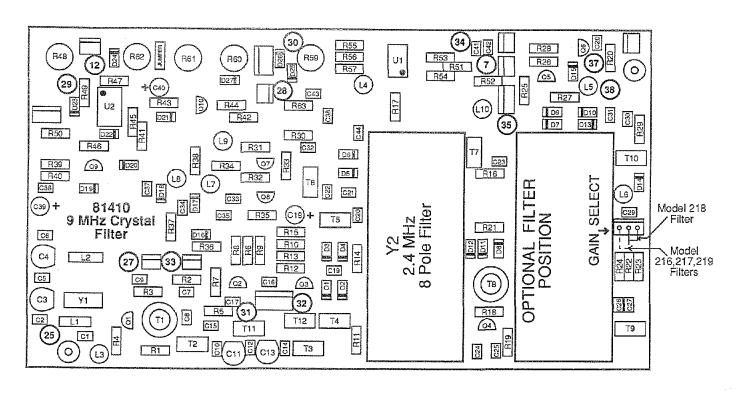
FIGURE 6-12. 81410 9 MHZ CRYSTAL FILTER COMPONENT LAYOUT
