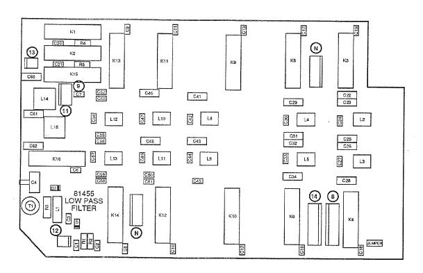
FIGURE 6-3. 81455 TRANSMIT LOW PASS FILTER COMPONENT LAYOUT
