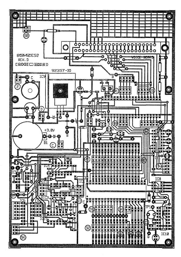
FIGURE 6-50. 81442 LOGIC BOARD CIRCUIT TRACE
