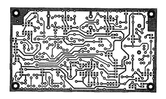
FIGURE 6-42. 81340 L. L. AMPLIFIER / NOISE BLANKER CIRCUIT TRACE
