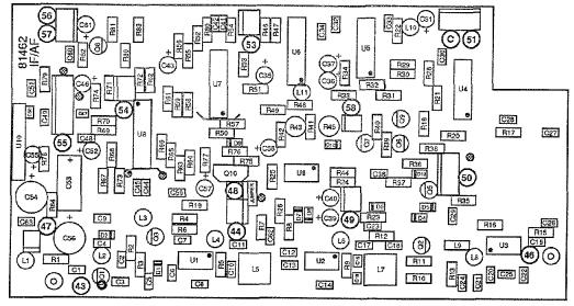
FIGURE 6-18. 81462 IF / AF BOARD COMPONENT LAYOUT
