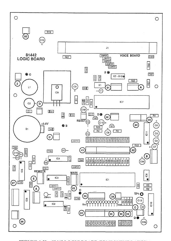
FIGURE 6-51. 81442 LOGIC BOARD COMPONENT LAYOUT
