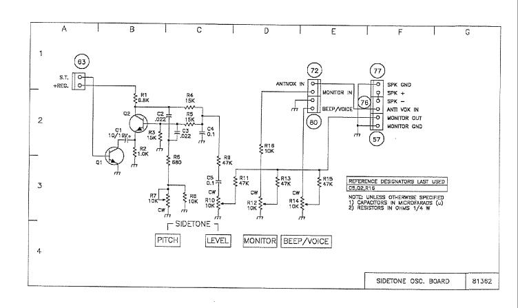
FIGURE 6-38. 81362 SIDETONE BOARD SCHEMATIC
