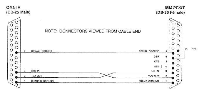
FIGURE 5-10A. IBM PC RS232 CONNECTOR CABLE
