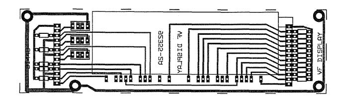
FIGURE 6-59. 81448 VF DISPLAY BOARD CIRCUIT TRACE
