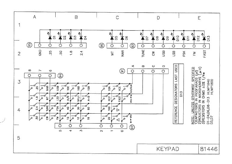
FIGURE 6-55. 81446 KEYPAD BOARD SCHEMATIC
