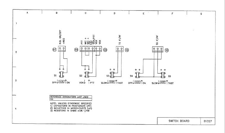
FIGURE 6-29. 81327 SWITCH BOARD SCHEMATIC
