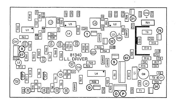
FIGURE 6-43. 81340 L. L. AMP. / NOISE BLANKER COMPONENT LAYOUT
