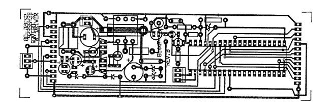
FIGURE 6-56. 81447 VF DISPLAY DRIVER BOARD CIRCUIT TRACE
