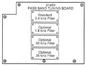
FIGURE 5-2. PBT CRYSTAL FILTER LOCATIONS
