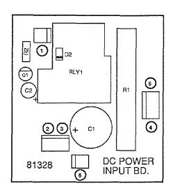
FIGURE 6-63. 81328 DC POWER BOARD COMPONENT LAYOUT
