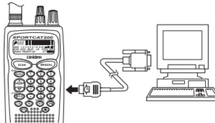
Plug the smaller end of the supplied remote interface cable into the remote port on the right side of your scanner.
