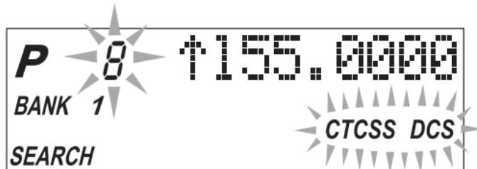
The scanner starts searching for an associated CTCSS tone or CDCSS tone when it stops on a transmission. All tones are checked if the transmission is long enough. However, if you press **(HOLD)**, and there is break before a tone is identified, the tone search starts where it left off when the transmission begins again.
