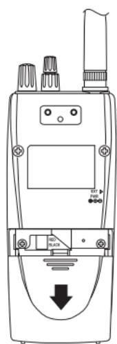
4. Carefully unplug the battery pack and lift it out of the case. You may need to exert slight pressure toward the top of the scanner as you slide the battery pack out of the case.
