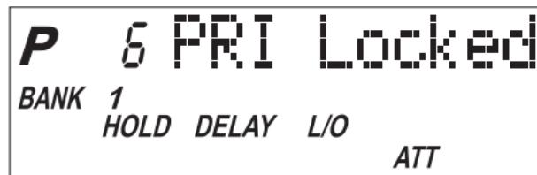
You can also remove **L/O** from all “Locked Out” channels in the selected Scan Banks (those appearing on the display.) Press and hold **L/O** for at least 2 seconds. You will hear 2 beeps and all channels except empty channels (000.0000MHz) are returned to the scanning cycle in the selected Scan Banks.
