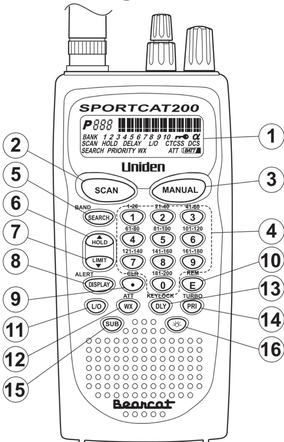
1. **LCD DISPLAY** — The liquid crystal display (LCD) shows the current channel and frequency. It also displays the mode, status, and bank indicators.
