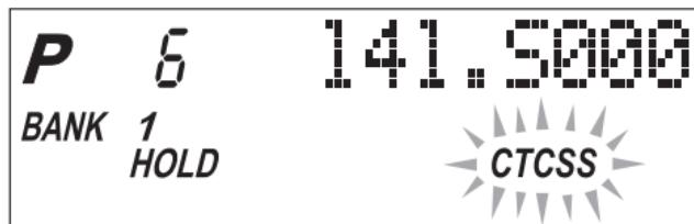
4. Press **E** to program the tone with the frequency stored in the channel.
