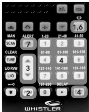
The scanner will monitor weather channels for alerts with matching FIPS codes. To exit SAME Standby mode, press **PRI/ALERT** again.
