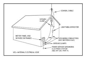
**WARNING:** Outdoor antennas must be properly grounded to prevent static buildup and lightning damage. Article 810 of the National Electrical Code, ANSI/NFPA 70, provides information about proper grounding of the antenna mast, connection of coaxial cable to an lightning arrestor, size of grounding conductors, location of the lightning arrestor and connection of grounding conductors to grounding electrodes.
