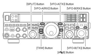
During Split operation, the VFO-A register will be used for reception, while the VFO-B register will be used for transmission. If you press the [**SPLIT**] button once more, Split operation will be cancelled.
