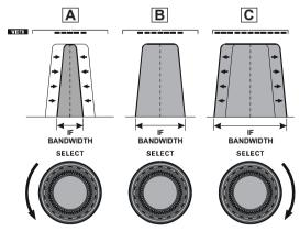
The default bandwidths, and total bandwidth adjustment range, will vary according to the operating mode:
