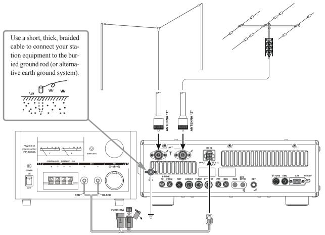
We recommend the use of the **FP-1030A** AC Power Supply. Other models of power supplies may be used with the **FT-950**, but the 13.8 VDC input voltage, 22-Ampere current capability, and DC cable polarity guidelines described above must be strictly followed.
