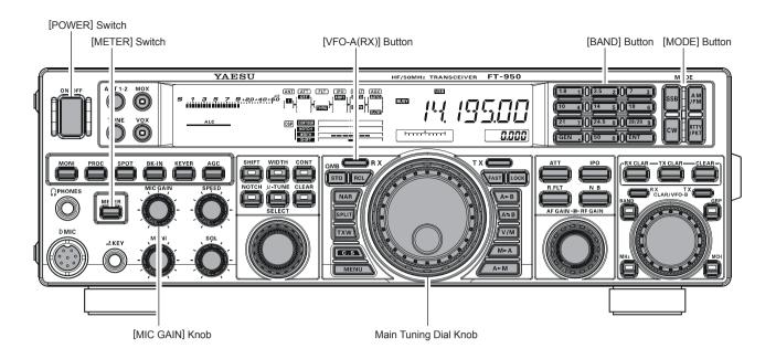
1. Press the **[BAND**] button corresponding to the Amateur band on which you wish to operate.
