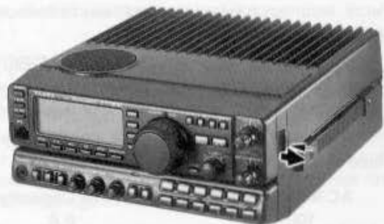
Removing the Front Sub-Panel
