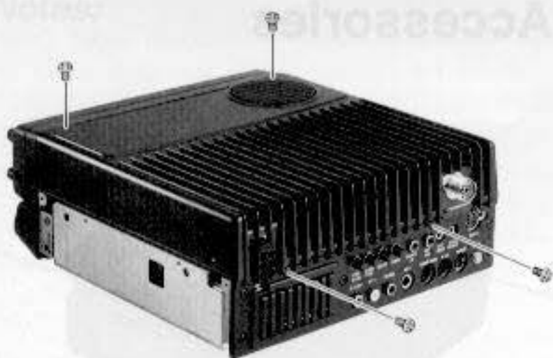
Fig. 4: Top Cover/Heatsink Removal
