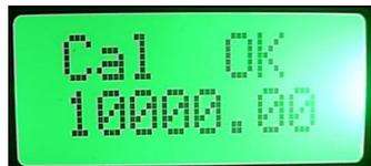
The 10 memory position will also be reset back to factory when you do the DDS calibration.
