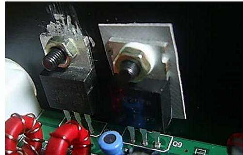
3. After installing all other parts, please install the the back cover and secure the Q9 and Q10, solder them to the PCB and cut the extra leads. Then secure the Q9, but use insulation pad and insulating washer then secure Q10, as above.
