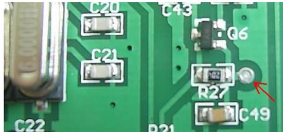
Now the frequency counter reading should be same as screen display (10000.00KHz), please adjust the tune knob if adjustment needed, pressing V/M/SAV for 2 second, the screen display below release, push V/M/SAV again to end.
