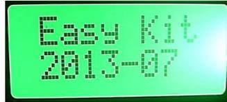
2. Waiting for 2 second, display change to below. Put your frequency counter to DDS testing point, the pad close to R27.
